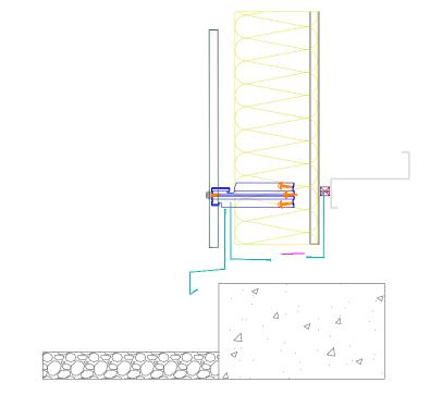
INSTALLATION NOTES - FLASHING JOINTS SEALED WITH BUTYL - FLASHING JOINTS FIXED AT 100mm CENTRES (RIVET OR STITCH) - FLASHINGS FIXED AT 450mm CENTRES - BRACKET MUST BE POSTIONED WITHIN 100mm OF END OF BAR OR MALE END JOIN
