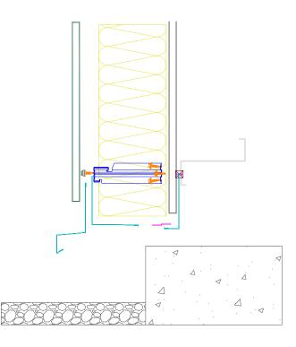
PROTEX APPROVED - INTERNAL CLOSURE FLASHING COATING - BRIGHT WHITE LINER GAUGE - 0.7mm
